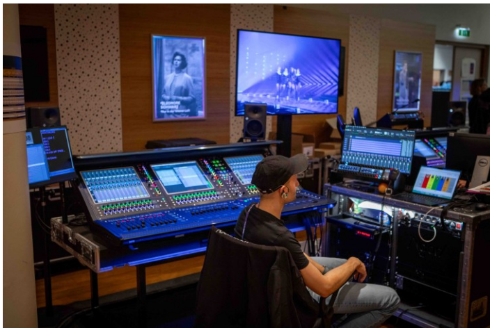
Failsafe operation was key at the ESC – one of two independent monitor consoles
